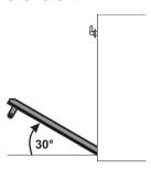
3. To reassemble the door, put the hinges in the relevant slots in the oven, making sure that grooved sections A are resting completely in the slots. Lower the door and once it is in place remove the pins from the holes in the hinges.
