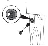
Cover the bushings with the covers removed previously.
