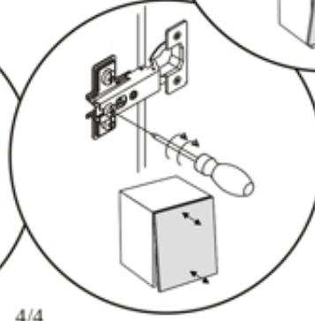
Attach the doors by clipping the hinges onto the hinge clips. Use a phillips head screwdriver to adjust the tilt and rotation of the doors to make them level.
