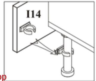
Adjust the feet to make the cabinet top level, then clip the toe kick into place.
