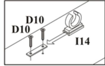
Screw on the toe kick clip brackets to line up with the cabinet feet and slide the clips on.
