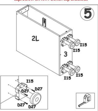
Carefully lay the cabinet down on a non-scratch surface. Screw on the feet with D27 screws.
