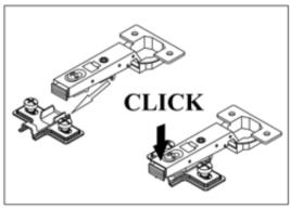
Attach the doors by sliding the hinges over the hinge clips, pushing down until they click into place.
