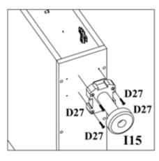
Carefully lay the cabinet down on a non-scratch surface. Screw on the feet with D27 screws.
