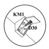
If required, screw on KM1 brackets for securing the bench top later on.
