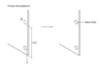
Drill out new hole for a tracking hinge
